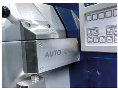
VC 460V features a new automatic lid lock system
